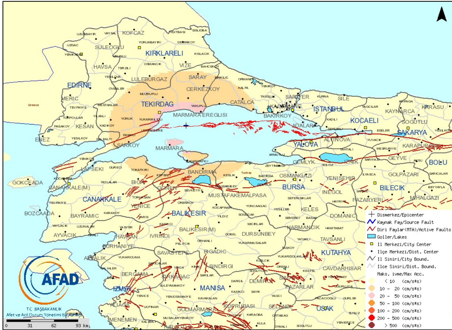
Fig.6: Peak Ground Acceleration Distribution of Marmara Sea Earthquake (Ml=5.1) (Çeken et al.2008)
